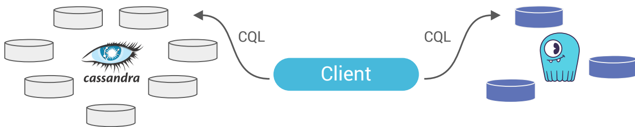
Dual Writes: Application logic is updated to write to both DBs
